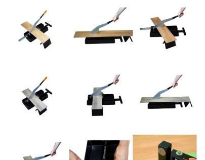
Fast and effortless cutting. No breathable dust. No noise. No sharpening required ever on blade. Removable stoppers to make angle cuts, cuts in length and wider than 230 mm planks. Max. width with stoppers : 230 mm overall. Cutting die with 2 positions : - Position 1 (narrow die) : to cut LVT (Luxury Vinyl Tile), HD vinyl and PVC floorings up to 12 mm thick. - Position 2 (wide die) : to cut laminate floorings up to 12 mm thick. Accessories : - 1 trestle.
