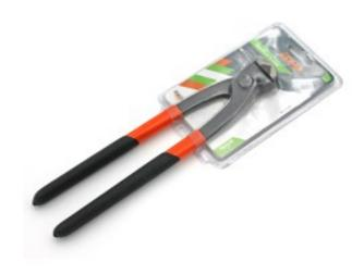
Forged tool made of chromium-vanadium (CrV). 55-61 HRC jaws. 42-48 HRC arms. Induction hardened jaws for greater performance. Handles with anti-slip PVC dipping.
