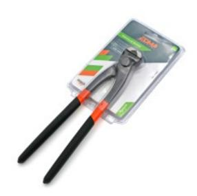
Forged tool made of chromium-vanadium (CrV). 55-61 HRC jaws. 42-48 HRC arms. Induction hardened jaws for greater performance. Handles with anti-slip PVC dipping.
