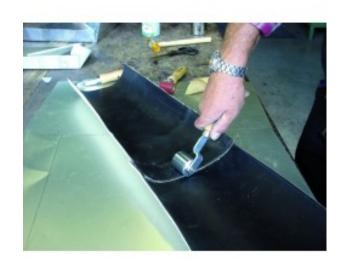
2 enclosed smooth-running ball bearings. Steel roller. Heavy duty design. Ergonomical wooden handle. For cold pressure welding. Ø 40 mm.
