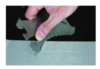
Stainless steel tracing template. Graduations from 5 to 100 mm (from 5 to 5 mm).
