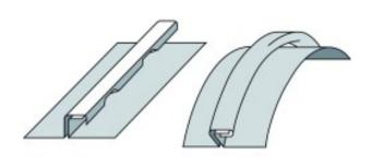
Tool joining prefabricated SPM-profiles. Used to tack up lengthwise beads to prevent withdrawal from folding press. Can make small radius lockseam without difficulty.
