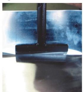
Lap joint. Raise large and deep measure. Folding depth : 175 mm.
