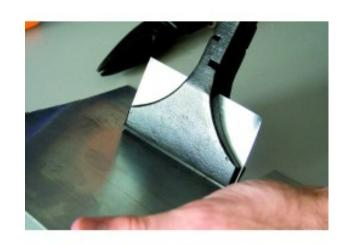
Lap joint. Handles with PVC dipping (thermal insulation). Folding depth : 66 mm.
