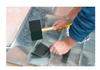
Forged steel. Block height: 25 mm. Long blade. Block with ø 5 x 15 mm hole.
