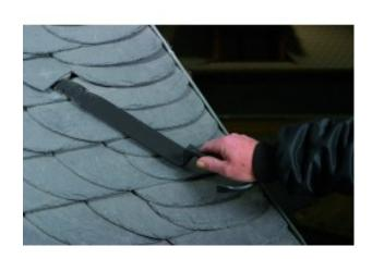
Traditional slate ripper. Welded. Made in steel.
