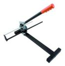
Clean cut = immediate bolting. No noise. Can be used to repair damaged rod. No metal scrap (no metal filings). No sparks - No risk of fire - No special permit. 545 mm adjustable cutting guide can be positioned on the right or left. Up to 6.6 soft steel : 60 kg/mm<sup>2</sup>. Cannot cut stainless steel threaded rod.
