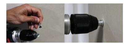
Depth stop to screw perfectly in plasterboards without drilling through them.
