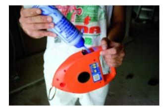
For long distance marking. Built-in filter system to prevent excess chalk. Rope diameter: 2,5 mm (braided). Capacity: 300 g.
