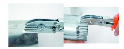
Pipe crimping tool for all types of metallic pipes. Swaging by 30 mm with 2 impressions in 1 press.
