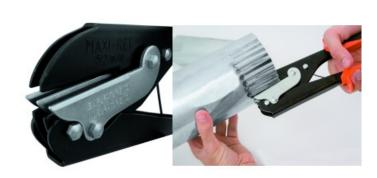
Pipe crimping tool for all types of metallic pipes. Special for stainless steel pipes up to 0.8 mm. Progressive reduction of the pipe diameter. Swaging by 52 mm with 2 impressions in 1 press.
