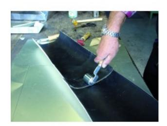
2 enclosed smooth-running ball bearings. Steel roller. Heavy duty design. Ergonomical wooden handle. For cold pressure welding. Ø 40 mm.
