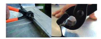
Seam and gutter opening pliers. Forged steel head. Head length 30 mm. Handles with PVC dipping (thermal insulation).
