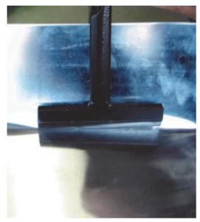
Lap joint. Raise large and deep measure. Folding depth: 185 mm.
