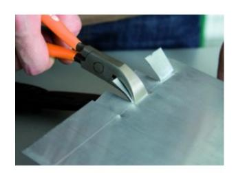
Lap joint. Handles with PVC dipping (thermal insulation). Folding depth : 28 mm.
